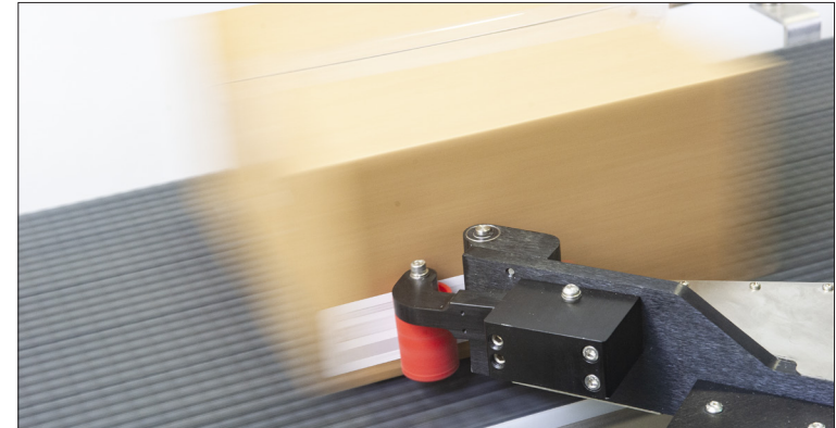
THE 258 APPLIES LABELS AT RATES OF 200 FT/MIN OR MORE, SO YOU CAN ACHIEVE MAXIMUM THROUGHPUT OF YOUR CASES OR TRAYS
