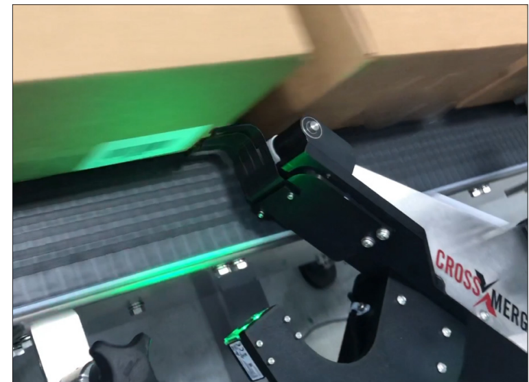
AN INTEGRATED SCANNER OPTION PROVIDES BARCODE VERIFICATION IMMEDIATELY AFTER LABEL APPLICATION
