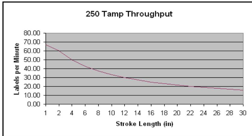
Line speed and product handling are a major factor in determining the ultimate throughput of labeled products. To obtain 60 PPM (products per minute) a 12" long carton would travel at 60 FPM. However, there must be a gap between products so that the product detector can sense the product and trigger the printer applicator to apply the label.
